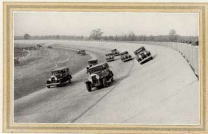
Where the sky is the limit on speed! One end of the four-mile speed loop which is used for a part of the breaking-in and durability runs of each car. The other parts of the runs are made up and down steep hills of gravel, dirt, concrete and brick
