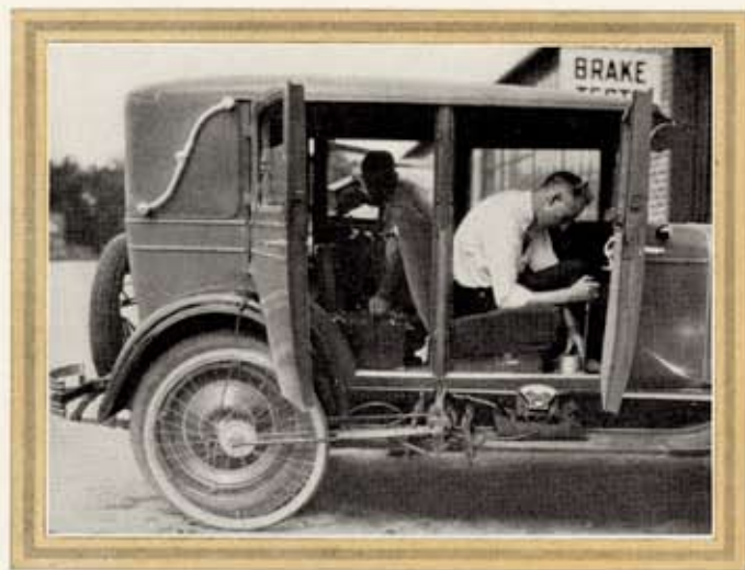
Preparing to measure vibration. This device, the telemeter, gives Proving Ground engineers an accurate vibration record at all speeds and under all driving conditions
