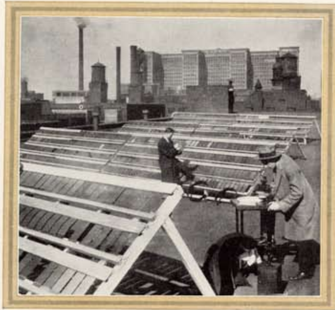
Panels finished in Duco are mounted on racks and exposed to the elements for years. Thus the Research Laboratories prove the durability of Duco under the action of sun, wind, rain, snow, dirt from city streets, and soot from near-by chimneys
