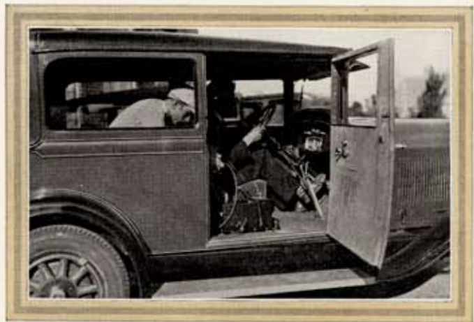
How quickly will a car stop? Good brakes mean safety and this instrument, the decelerometer, gives the Proving Ground valuable information and points the way to even better brakes in General Motors cars
