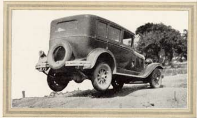
Ride 'im cowboy! Besides the miles of good paved and gravel roads at the Proving Ground, there are some highly uneven roads for spring tests. It was not just left to nature to make these roads bumpy. They were carefully laid out and built by engineers and are of various degrees of severity
