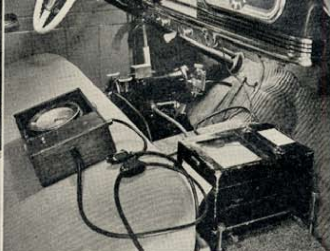
• Mounted behind the fifth wheel speedometer, the little black box precisely measures the stopping distances in the hundreds of braking tests. Right:—The chronometer (on the seat) times the brake machine (rear) powered by compressed air as it depresses the brake pedal exactly at the pressure desired. The recorder (right) marks on tape deceleration time, pedal pressure and pedal travel required to stop the car.
