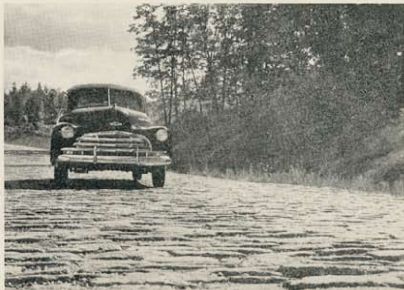
• One of the world's roughest rides, the "Belgian Block" road of heavy granite blocks laid unevenly.
